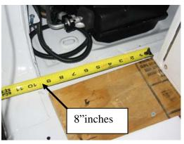
Measurement from driver-side **Rear Doorframe** to vehicle doorframe shown above
